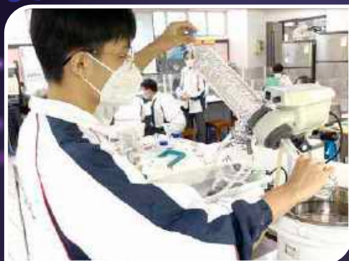
A student conducts an experiment on fat content in potato chips using the rotary evaporator.
